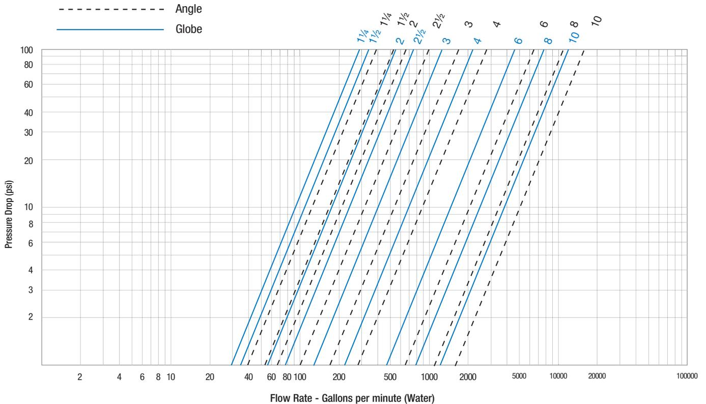
The  $C_V$  factor of a valve is the flow rate in US gpm at 60° F that will cause a 1 psi drop in pressure. The factors stated are based upon a fully open valve.
