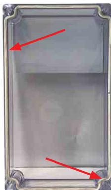
9. Using a #2 Phillips head screwdriver, reinstall the four screws that secure the cover of the Cellular Gateway.
