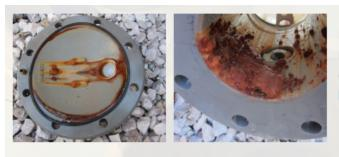
In these images taken 14 months after installation you can see many of the tubercles common to MIC and extensive corrosion.
