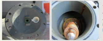
These images taken after 16 months in the same application as above shows little to no corrosion. Any corrosion resulting from a breach in coating has not spread.
