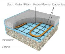
Install RadiantPEX+ in slab systems for radiant floor heating applications.
