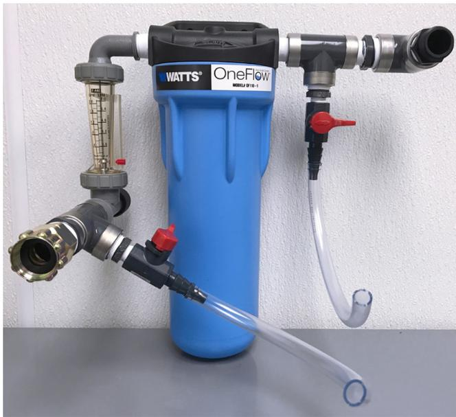
Figure 2. SSI Testing setup
