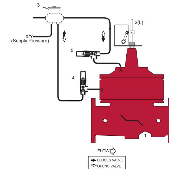
controlled by the adjustable opening speed control, which restricts the speed at which fluid and pressure evacuate the cover chamber. When the valve reaches the full open position, the limit switch is actuated, turning the pump off.
