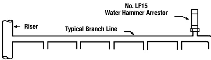
As shown, it has been established that the preferred location for the water hammer arrestor is at the end of the branch line between the last two fixtures served.
